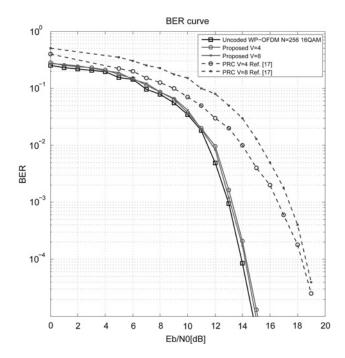
**Fig. 9** *BER performance of the proposed WP-PTS-ESID scheme, compared with the PRC scheme* [17], *for* V = 4 *and* 8
