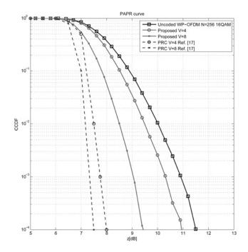
**Fig. 8** *CCDF of PAPR for the proposed WP-PTS-ESID scheme compared* with the PRC scheme [17], for V = 4 and 8
