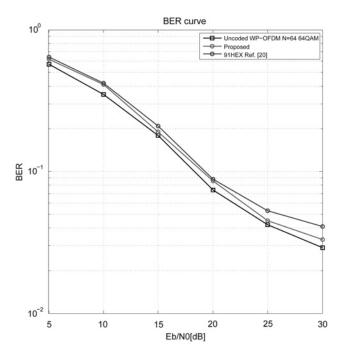
Fig. 11 BER performance of the proposed WP-PTS-ESID scheme compared with 91-HEX [20] under a Rayleigh fading channel
