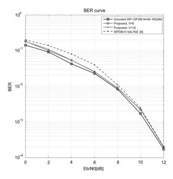
Fig. 13 BER performance comparison between the proposed WP-PTS-ESID scheme and the related work of wavelet packet tree pruning scheme [6] with corresponding I = 6 bits
